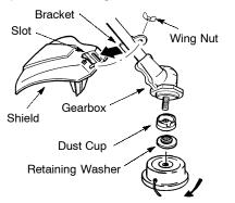
**NOTE:** Make sure all parts are properly installed as illustrated in the illustration before installing the trimmer head.
